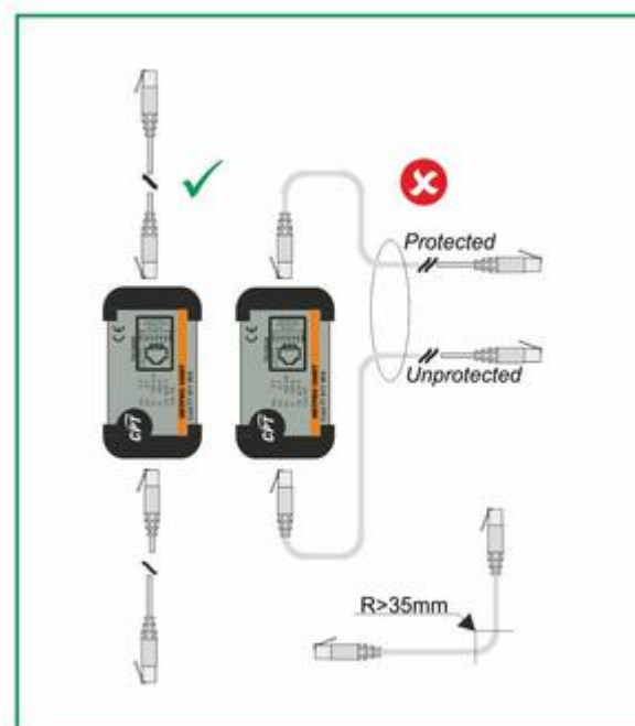
Wiring diagram
